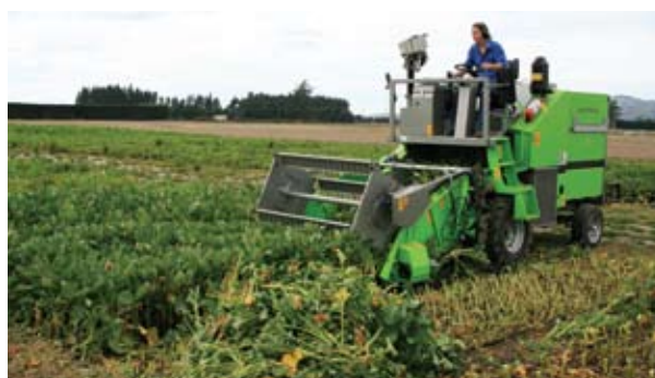
Total forage yield of each breeding line is mechanically harvested and individual plant measurements like plant height and leaf to stem ratio is recorded.
